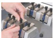
All pieces of this machine that are contacting with test sample are made from stainless steel or aluminium and strong enough to avoid bending during test.
