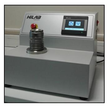
**Purpose** – Determination of distension and strength of the leather grain or finished surface and the last ability of uppers assembly irrespective of material, to assess the suitability for the end use, according to the standards EN ISO 3379; EN ISO 17693; EN ISO 17695; TM 24.
