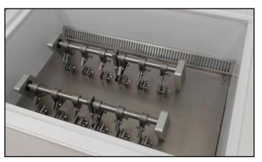
After all samples are clamped, the counter is set with a number of flexing cycles. At the set cycles, the machine stops automatically, and the samples are visually assessed, and any damage is recorded.
