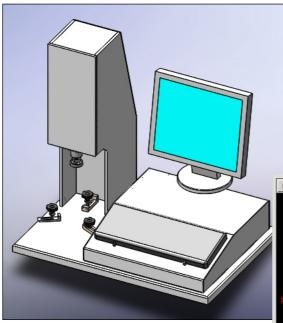
**<u>Purpose</u>** – Evaluate the shock absorption properties of materials or assemblies of footwear bottom, according SATRA TM142.
