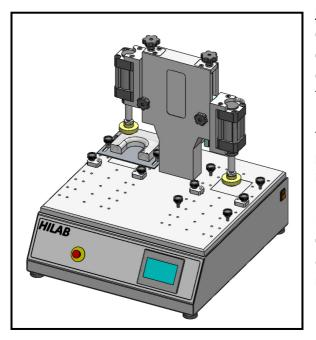
**Purpose** – Evaluate the structural behavior of the sole unit or sheet material when submitted to a repeated compression. This method simulates what occurs in the heel of a sole during footwear wearing, according to SATRA TM156.
