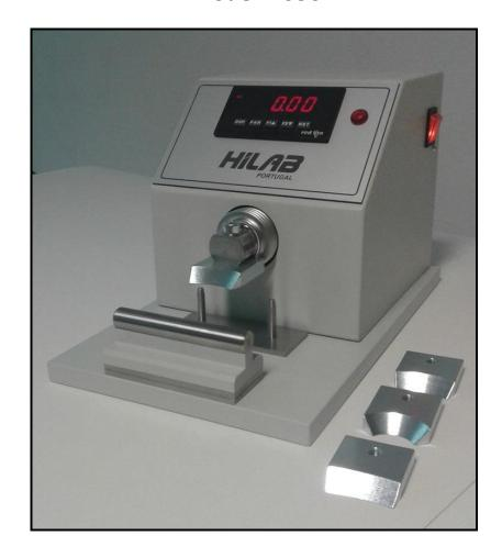
**Purpose** – Determine the adhesion resistance in toe and heel, according to test method TM 404.
