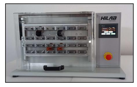
**Purpose** – assessing the resistance of rubber upper materials to damage by repeated flexing., according to **EN ISO 20344:6.5.2.2**
