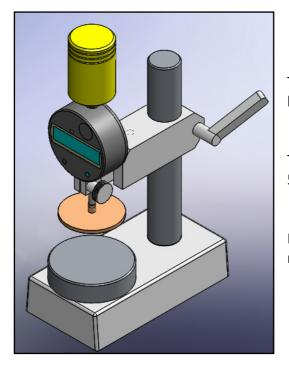
This measuring system is composed by digital gauge with high accuracy.
