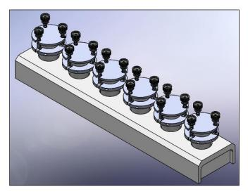
**Purpose** – Determining the water vapour absorption on leather and non-leather used in gloves, according EN ISO 21420.
