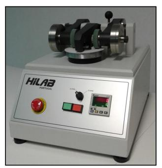
**Purpose** – Determine the abrasive wear resistance of leather, coated materials, textiles, and fabrics, to assess the suitability for the end use, according to ISO 17076-1; ISO 5470-1; ASTM D-3884.
