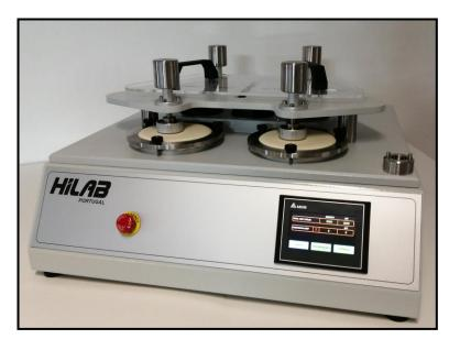
Purpose The present equipment "MARTINDALE Abrasion Machine" intended to determine resistance of a material to wet and dry abrasion and it's mainly applicable to fabrics, coated fabrics and leathers but it can be used with any flexible sheet material used for footwear, clothing, gloves and many other products, according to ISO 12947-1; EN ISO 5470-2; EN ISO 20344:6.12; EN ISO 17704; EN ISO 12945-2; TM 31.
