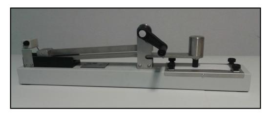
This equipment consists of a base on which the test sample is fixed. A sliding mechanism is arranged to traverse a finger along the sample.
