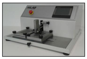
**Purpose** – Assess the resistance of upper and glove materials to be cut by blade, according **EN ISO 20344:5.23; ISO 23388:6.2; EN 388:6.2.**
