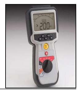
Purpose – Assess the electrical insulation of footwear, according EN ISO 20344:5.13; IEC 61340-4-3.
