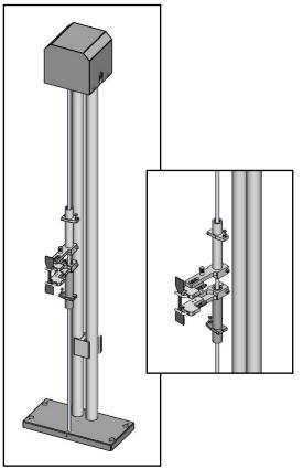
An Extensometer can be installed to assure higher accuracy in distension measurements. Normally required for polymeric materials or other, according to standards requirements. In case of use of extensometer, the test method is configurated to
