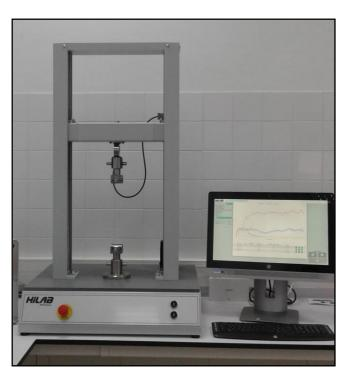
**Purpose:** Perform tensile, compression, flexure, bend, shear, and cyclic tests.
