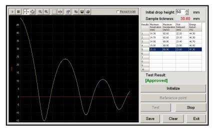
The equipment is controlled by a PC which runs specific software allowing configuration of the type of tests and showing graphically the displacement, time, force, energy, deceleration, energy return, rebound height and test results, according to the requirements of each standard. All tests are stored in a data base allowing future analysis and re-analyze.
