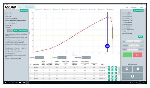
During test, a graphic is generated showing in real time the behavior of the sample.
